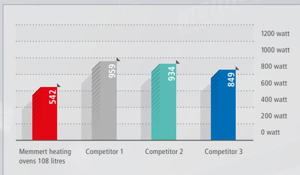
Heat emission at 250 °C, air flap closed
