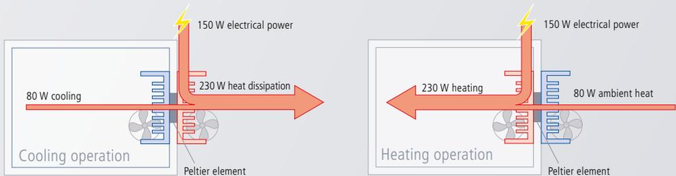
In contrast to compressor technology, Peltier technology works in a particularly economical and energy-saving manner at temperatures close to the ambient temperature, since energy is only required if heating or cooling is needed. Heating and cooling are perfectly fine-tuned.
