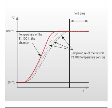
The setpoint wait function ensures that the sterilisation time is exactly maintained in the Memmert hot-air steriliser
